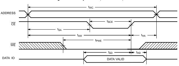
Figure 6. Write Cycle No. 2 (CE Controlled) [16, 17]
